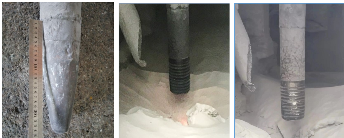
(a) Q235 steel breaker after 6 months.
